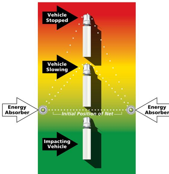
CatchNET's energy absorbers use a patented "metal bender" principle for absorbing energy, which provides the means to stop vehicles of varying weights and speeds. The absorbers are primarily comprised of a chamber, a length of metal tape and a series of offset pins.
