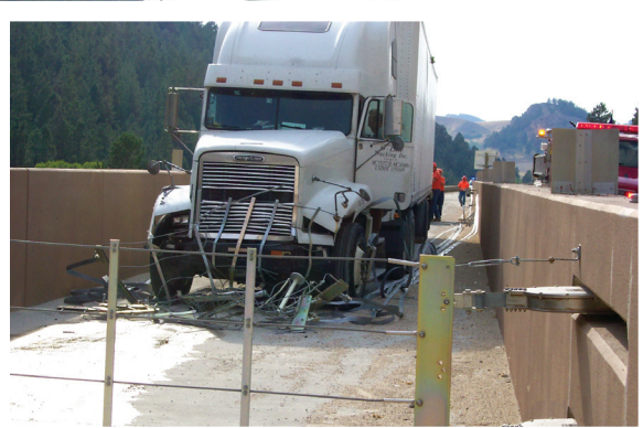
Used CatchNET August 26, 2010. No injuries, minimal damage. 15,000 lbs, 60 mph, used 1 net.
