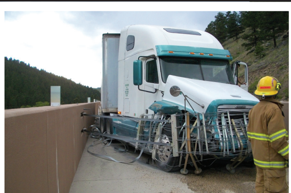
Used CatchNET August 26, 2010. No injuries, minimal damage. 15,000 lbs, 60 mph, used 1 net.
